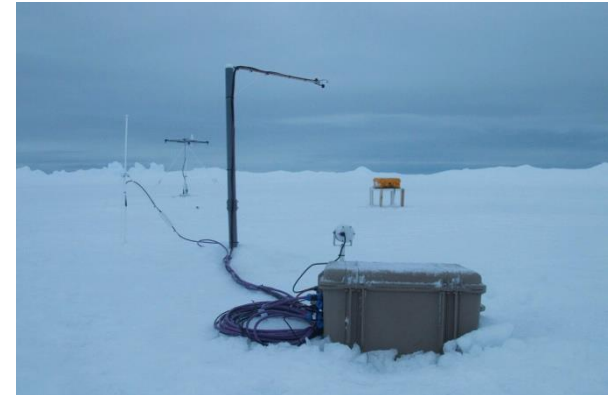
Modular sea ice buoy consisting of the main control unit (grey box) a mast structure (grey pole) and a thermistor chain mounted on a tripod (white). In addition, the photo shows a Snow Buoy and a thermistor string buoy in the background.
